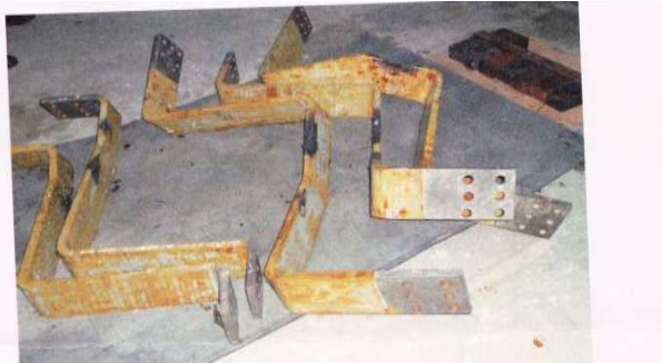
Photos of Generator terminal lead Bar
