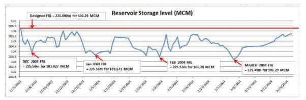
Figure 46: Reservoir Operation Simulation during 1 Dec 2003 – 31 March 2004
